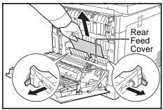
If a paper jam has occurred inside the machine as shown, open the rear feed cover and pull out the paper.
